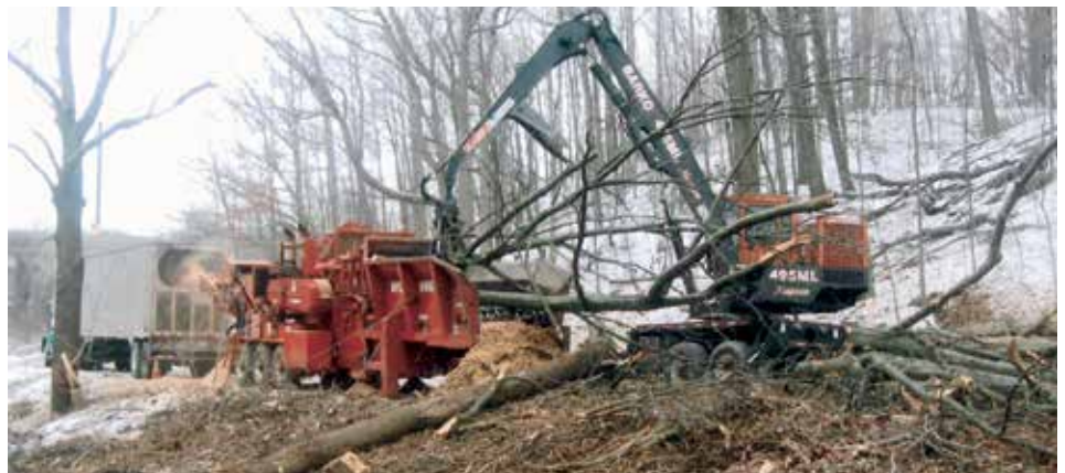
ROAD and building expansion requires increased space, in many cases needing equipment such as log loaders with grinders to clear that space.
