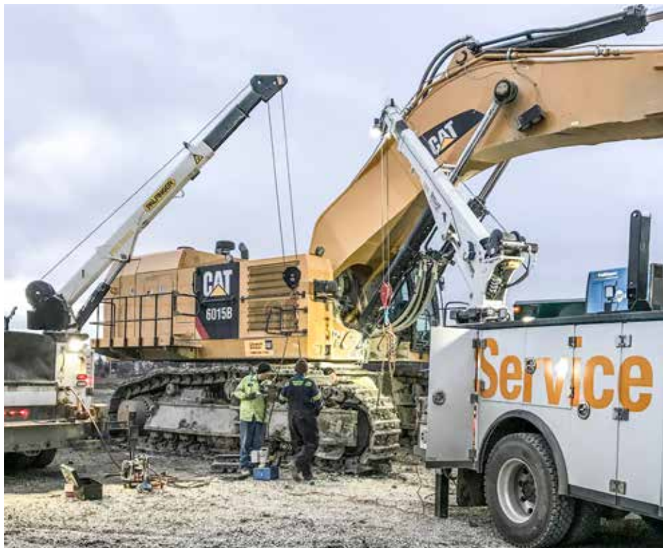
Ohio CAT and Trumbull mechanics repairing an idle roller.
