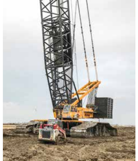
WALKING their Liebherr 1750 on the Timber Road IV Windfarm in Paulding County is Kiewit Power Constructors.
