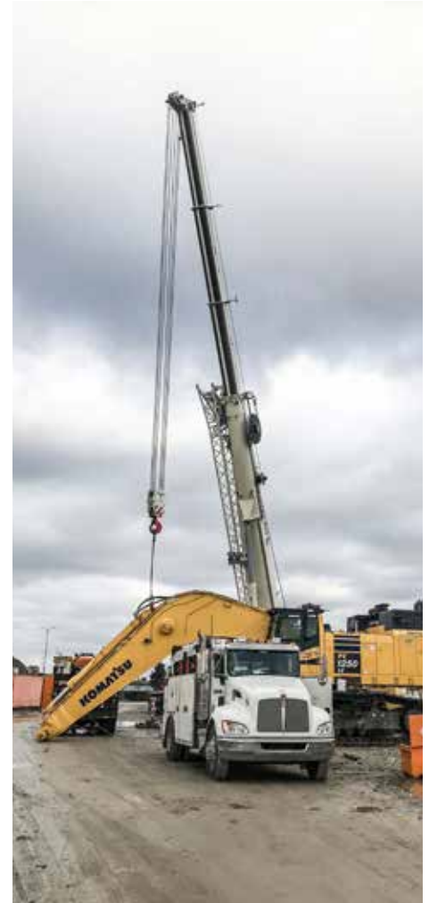
ASSEMBLING a Komatsu 1250 on the DiSalle Bridge project in Toledo are Kokosing mechanics.
